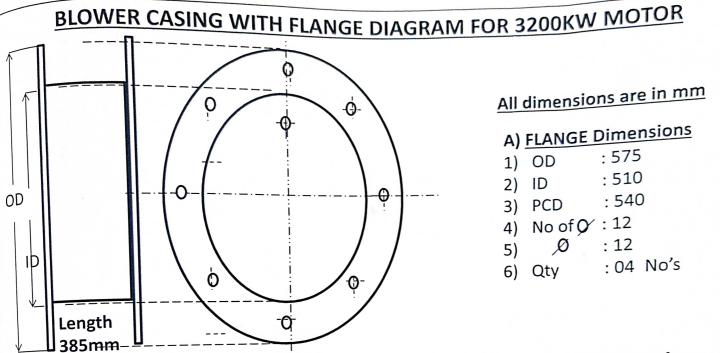
ASPECIFICATIONS: High Efficient Cooling Blower Unit with complete casing, grill, fan and motor, . for 3200kw Ht motors Make, Type: IGH5254-02H, SRIM should have the following specifications:
