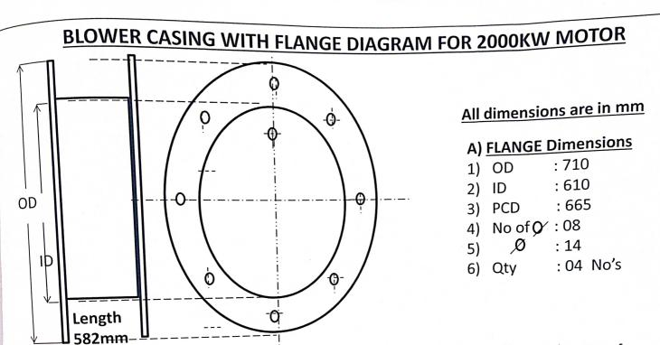
A SPECIFICATIONS : : High Efficient Cooling Blower Unit with complete casing, grill, fan and motor, . for 2000kw Ht motors Make, Type: IGH5254-02P, SRIM should have the following specifications:
